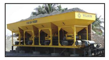
hopper design has been accurately calculated to allow constant discharge of aggregate without bridge formation and plugging.
