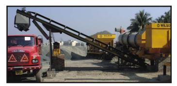
at discharge end of the conveyor driven by AC Motor coupled with SMSR Gear Box. The Hydraulic Dual gate hopper open via Cylinder powered by a compact Power Pack. The operation is automatic duly controlled from AC Panel. Hopper consist scrapper for cleaning the Load-Out Belt properly and assuring falling hot-mix material in to hopper.
