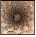
The Wilson Thermo Drums come in various sizes ranging from 20 TPH to 120 TPH. All thermo drums are made of 10-12 mm thick heat and wear resistant steel plates.
