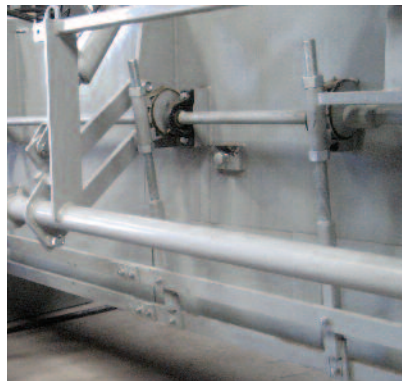
Tamper bar and vibrator mount/lift.
