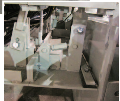
Everything works together to create pavement with a smooth flat finish with a sharp edge (top). Edge overbuild feature compensates for edge slump (bottom).
