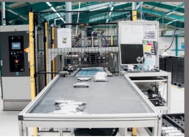
Automatic machining line for pistons for AC compressors with 6 TSUGAMI lathes, robotized unloading system, conveyors, washing machine (monthly capacity 270 000 pcs, to double next years).
