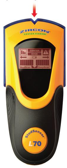
The StudSensor™ L70 OneStep® quickly and easily locates the center, edges, and direction of wood and metal studs while also alerting you to the presence of live AC electrical wiring. It features a bright, backlit LCD display and a low battery indicator informing you when your battery should be replaced for optimum performance.
