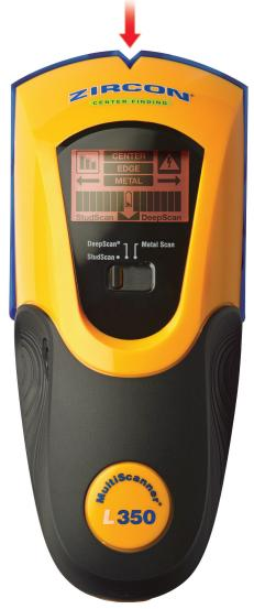
The MultiScanner<sup>®</sup> L350 OneStep<sup>®</sup> quickly and easily locates the center, edges, and direction of wood and metal studs and joists behind walls, floors, and ceilings. It also locates metal targets up to 3 in. (76 mm) deep. A 3-mode switch makes it easy to change modes, while the ultra-bright display screen, SpotLite<sup>®</sup> Pointer, and audio tone all indicate the location of the target. The signal strength indicator helps to distinguish between shallow and deep targets.
