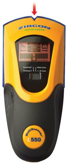
The MultiScanner® L550 OneStep® quickly and easily locates the center, edges, and direction of studs and joists behind walls, floors, and ceilings. It also locates metal as well as live AC electrical wiring. A 4-mode switch makes it easy to change modes, while the ultra-bright display screen, patented SpotLite® Pointer, and audio tone all indicate the location of the target. The signal strength indicator helps to distinguish between shallow and deep targets.
