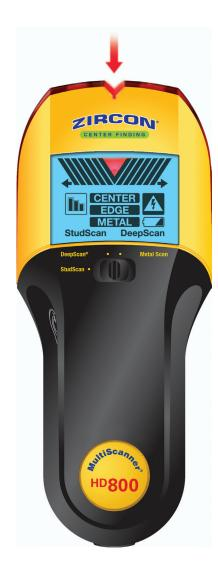
MultiScanner® HD800 quickly and easily locates the center and edges of wood and metal studs and joists behind walls, floors, and ceilings. It also locates metal targets up to 3 in. (76 mm) deep. A 3-mode switch makes it easy to change functions, while the backlit display screen, SpotLite® Pointer, and audio tone all indicate the location of the target. The signal strength indicator helps to distinguish between shallow and deep targets.
