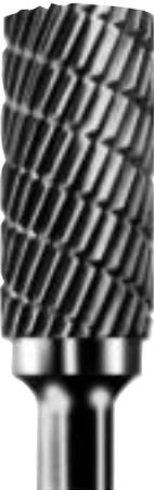
Standard cut with chipbreaker. Used for tempered, unhardened steel, cast steel and weld seams.
