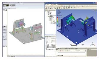
Static structural analysis of a production fixture using SpaceClaim and ANSYS.
