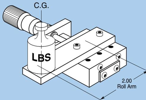
A 2 pound load is mounted to a single axis linear stage. The diagram shows the load's position in reference to the positioner carriage center. This shows that the load is offset 2 inches from the carriage center creating a roll moment.
