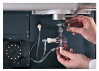
**Simple installation** The Multimode Sample Introduction System (MSIS) is easy to plumb, install and operate.
