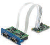
PCM-24D2R2/ PCM-24D2R4 OXPCIe952 UART, Isolated RS-232, RS-422/485, DB9 x 2 • 2000 V oc isolation protection • RTS/CTS/Xon/Xo flow control
