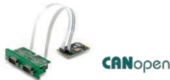
PCM-26D2CA SJA1000 CANBus, CANOpen, DB9 x 2 • CAN 2.0 A/B • 1Mbps, 16MHz
