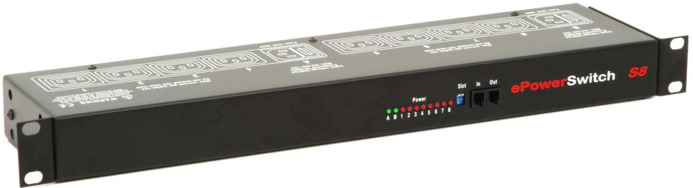
**ePowerSwitch-S8 (Slave)** is a power distribution and control unit that enables power management of 8 devices through a RS232 serial connection. The controlled power outlets can be extended up to 32 by cascading up to 4 Slave models. This ePowerSwitch is ideal to control power through the serial connection of a PC, a KVM switch or a Console Server.
