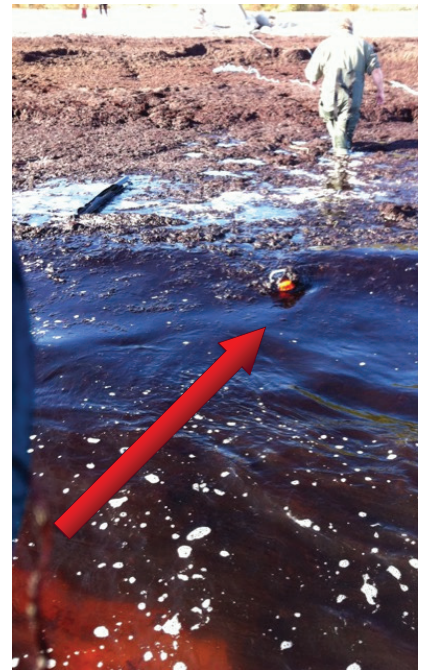
Fig 1: SeaGuard® RCM (with CTD & O 2 ) being installed to estimate degree of algae decomposition before harvesting in biogas production project
