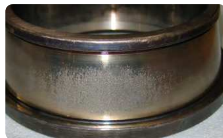
Surface initiated fatigue on the inner ring raceway of a tapered roller bearing
