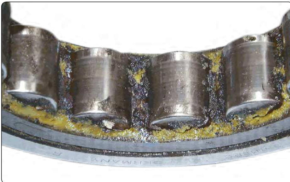
Lubricant degradation Black discoloured grease on the cage bars caused by passage of current
