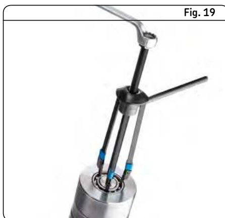
SKF deep groove ball bearing puller
