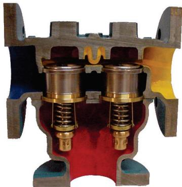
When the liquid reaches a predetermined temperature, the elements open and divert the flow to a different port. Liquid flows from yellow to red and is diverted to blue once the predetermined temperature is reached.
