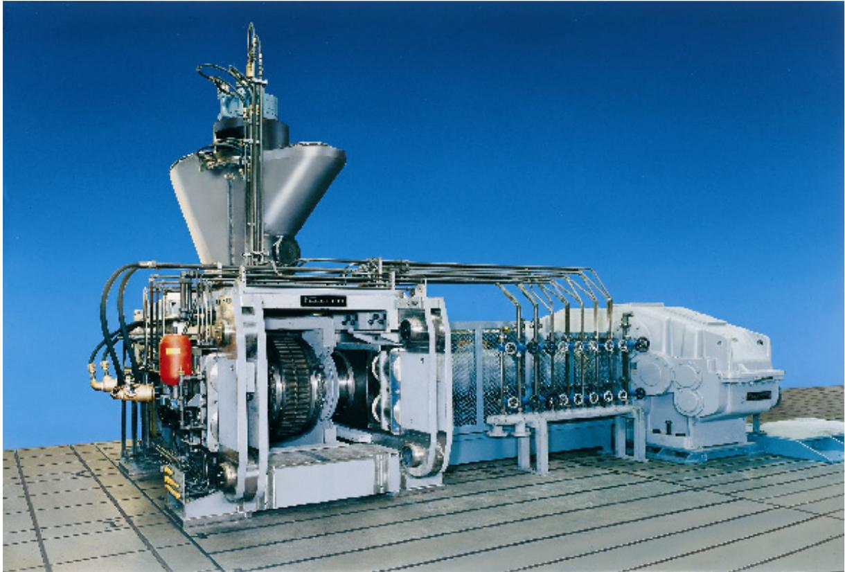
Figure 4: *Briquetting machine for DRI from pellets and lump ore
