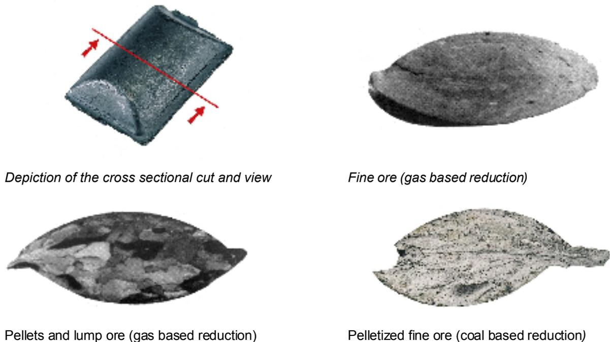
Figure 9: Cross sections through briquettes made with material from different direct reduction processes.
