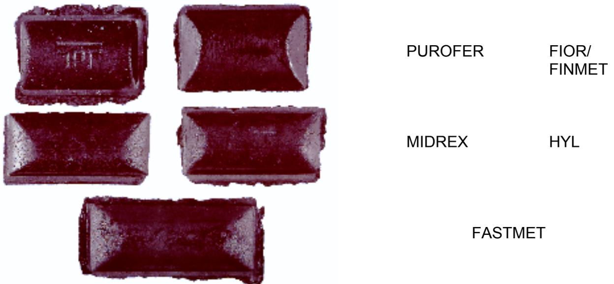
Figure 8: Briquettes made of product from different direct reduction processes by hot briquetting.
