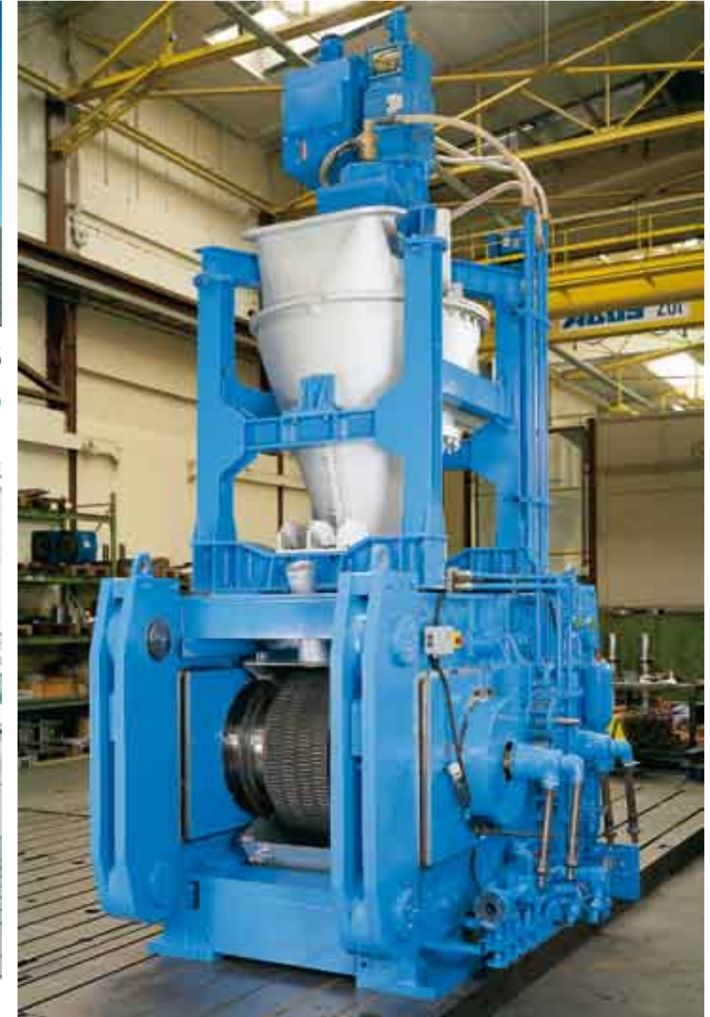
Press type 72/8 for briquetting of magnesium oxide (design temp. 450°C)
