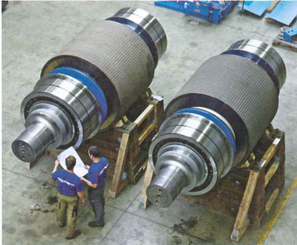
a roll diameter of up to 2000 millimeters and in this way, for example, they can make possible throughputs of more than 1200 metric tons per hour for the cement industry. SKF developed a special self-aligning roller bearing in the Explorer performance class (see box) for this application.
