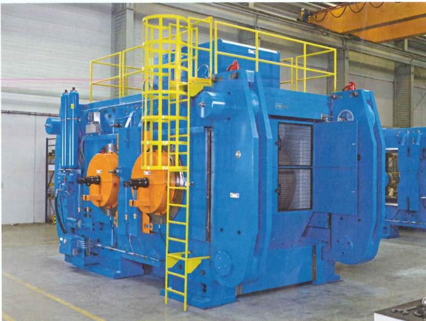
2 Each roll consisting of a core, tire and 2 self-aligning roller bearings has a diameter of 1800 mm and weighs 52 700 kg. The bearings have a bore diameter of 850 mm and weigh 2900 kg
