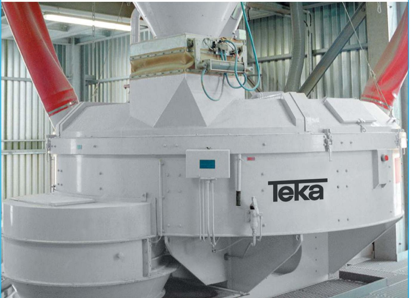
TEKA turbine pan-type mixers THZ are pan mixers for batching operations, and are available in sizes from 250 to 6000 liter filling capacities.
