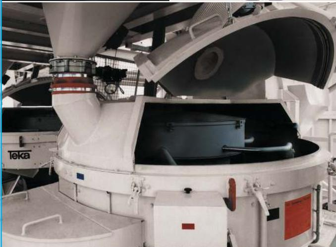
Large, hinged segments with variable positioning are possible, raised and lowered by a manual- or motorized cable winch.
