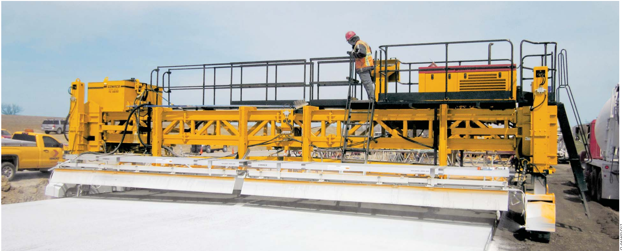
The T/C-5600 texture/cure machine is capable of tining and curing in a single pass. It can be set up for either transverse or longitudinal tining and spray.
