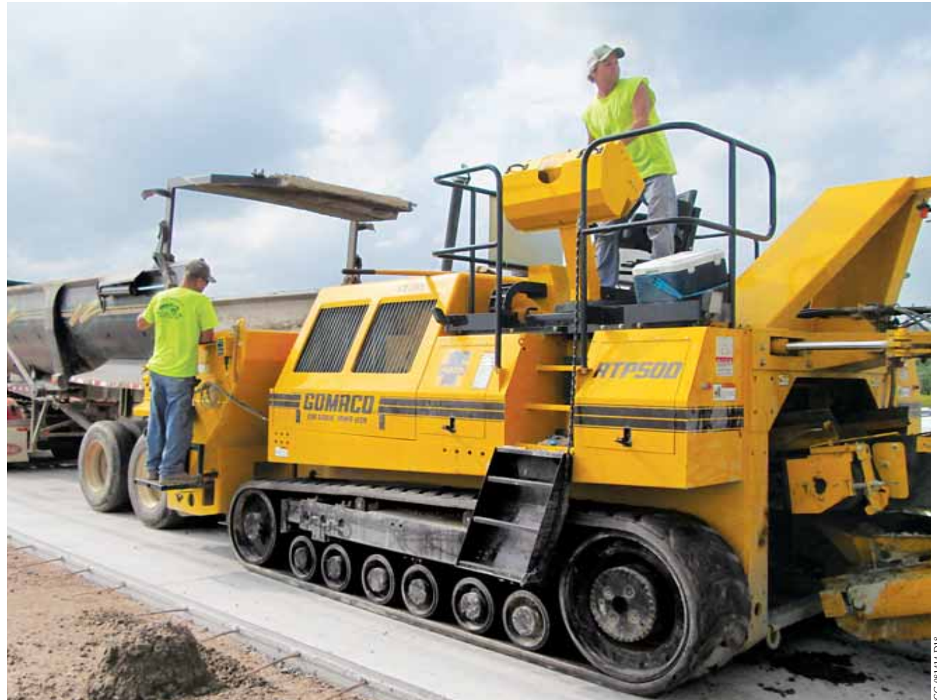
The operator's console can move to provide the operator with a panoramic view of the whole placing operation.
