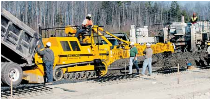
The RTP-500 with its 19 inch (483 mm) wide and 13.5 feet (4.11 m) long rubber placer tracks can traverse any terrain to get the job done.
