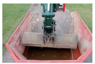
For attachments and buckets weld plant numbers and company logos/ details to aid identification.
