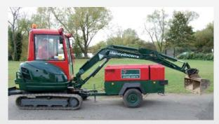
When leaving equipment overnight on sites secure compressors under boom arms of mini excavators then use immobilisers or hydraulic locks to prevent removal.
