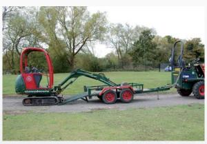
Make the thiefs life harder. Equipment removed from trailer and boom arms extended and immobilisers and /or hydraulic locks set preventing ease of theft.
