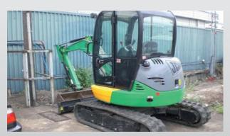
Stolen JCB 8012 found North London September 2009. Note the scratched triangular panel behind door where CESAR registration plate ground off. Officer instantly identified equipment using RFID tags hidden within equipment. Machine valued at £12,000 returned to owner without cost.
