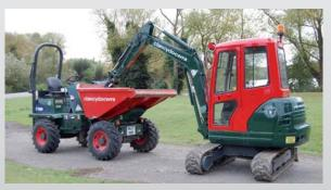
Secure equipment together preventing either being lifted or dragged away. Use immobilisers and/or hydraulic locks with chain and padlocks.
