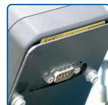
Serial port for downloading data
