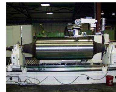
Oven roller for continuous annealing, ball-shaped mould to customer specification
