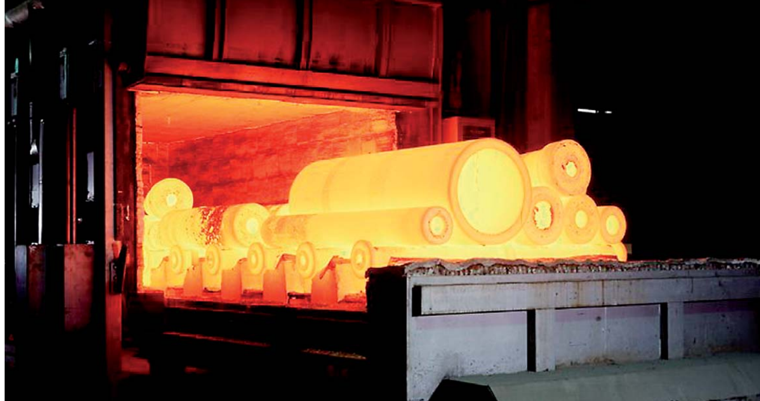
Tubular supports in a heat treatment oven
