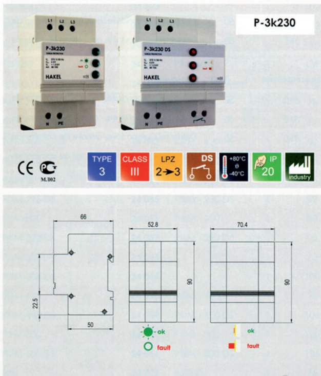
Three MOV + GDT surge arrester
