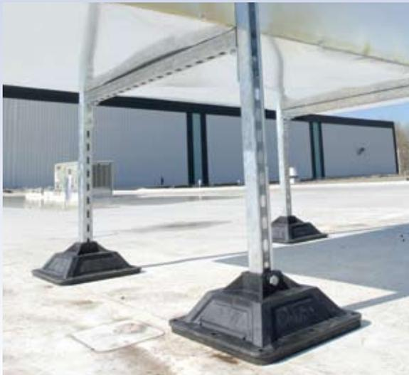
**The CADDY® PYRAMID RPS H-Frame Series Support System** is designed to provide superior support for pipe, conduit, ductwork, cable tray or any combination of these without causing damage to the rooftop membrane. The base is made from recycled, UV-stabilized engineered thermoplastic and features a highly engineered design to help uniformly distribute the load.
