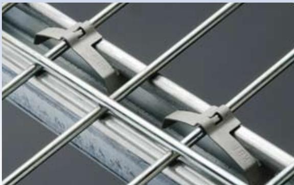
**The KBT Wire Basket Tray Clip** is an easy-to-install, time-saving solution for securely attaching wire basket tray to strut. Simply place the basket tray on top of the strut, position the KBT clip over the tray at the desired position, squeeze and slide it in place to finish the connection – it’s that simple!
