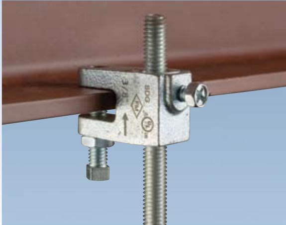
**CADDY® ROD LOCK** provides a quick and economical solution for installing electrical and mechanical systems supported by threaded rod. The system includes the CADDY ROD LOCK beam clamp, channel nut and an anchor screw. The SN Series Nut can also be used as an accessory to the system.
