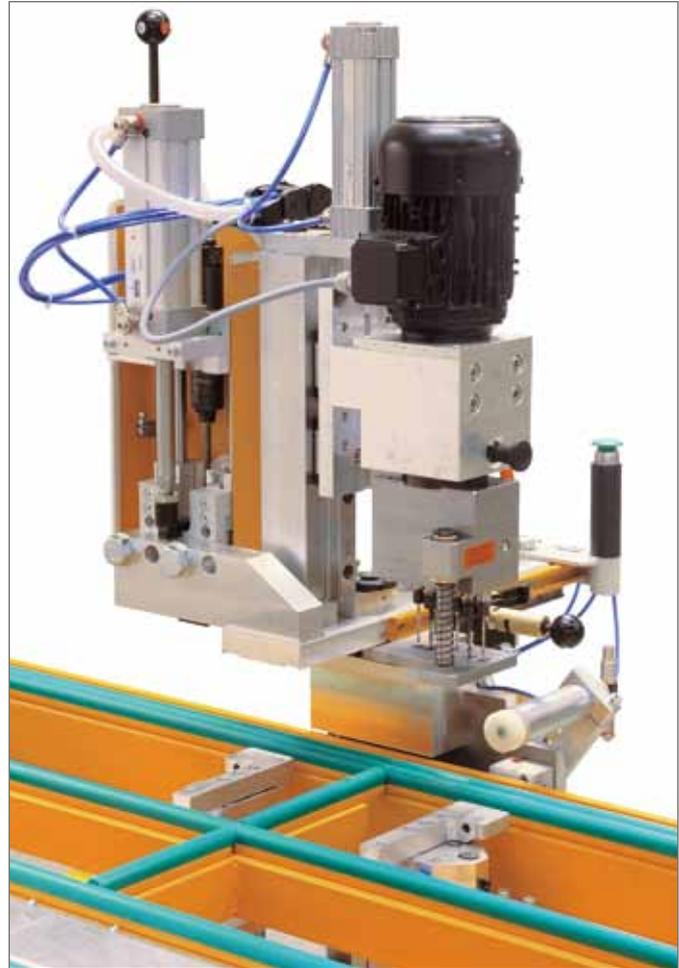
*Two pneumatic fold stops that are lowerable below table height with a rotary turret for the exact positioning of two to four different frame construction depths*
