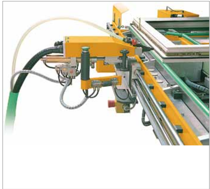
Manually controlled feed screwdriver with automatic screw feeder and attachment of fittings or special fittings
