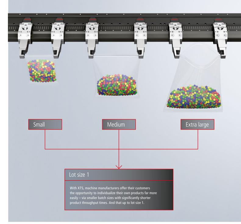
line efficiency for the owner. And with the XTS's Track Management software functionality, you can split the XTS system into individual, physically separate sections to do things like inserting or removing movers. You can thus carry out tool changes or maintenance activities without having to interrupt the regular production flow.
