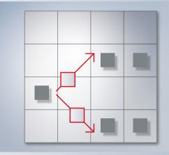
**Dividing:** Simple flow division, e.g. diversion of a product flow into several channels
