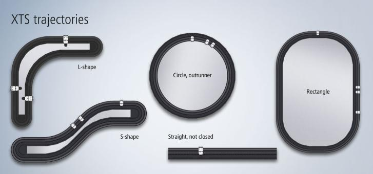
The XTS motor modules can be combined as desired.
