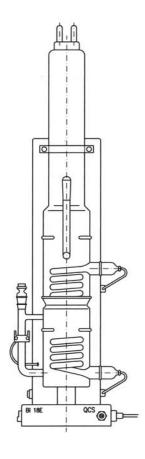
In the Bi 18 E components coming into contact with water are quartz glass parts which, contrary to ordinary laboratory glass is non-hygroscopic and thus resistant to H2O. These properties warrant the high purity requirements a distillate must fulfill.
