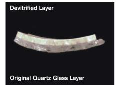
High cristobalite has nearly the same density as glassy silica and thus cannot be seen on the surface. However, upon cooling, high cristobalite undergoes a structural change from a cubic to a tetragonal crystal structure at about 275°C. This is accompanied by a large decrease in density that can result in some cracking and spalling. Refractive index differences resulting from the birefringent tetragonal crystal structure also cause the devitrified spots to turn white.
