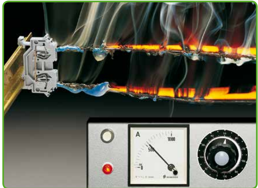
Test arrangement: "Short-Time Current Withstand Test"
