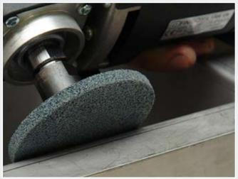
Smoothing of drilled, punched or milled openings
