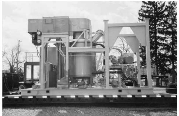
Self-contained batching/mixing skid.
