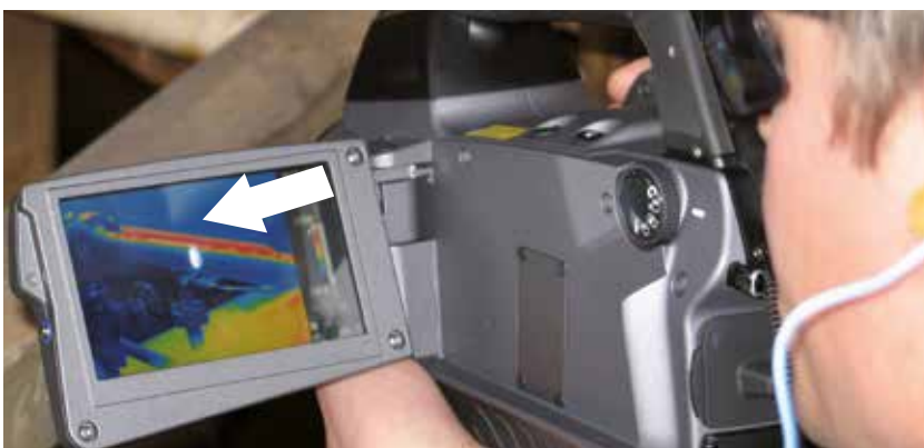
Real-time image of a gas leak displayed on the built in LCD screen
