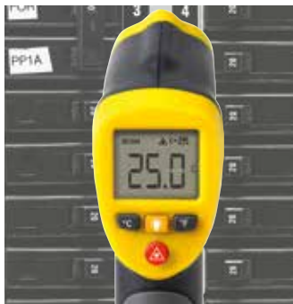
IR thermometer, temperature measurement in one spot
