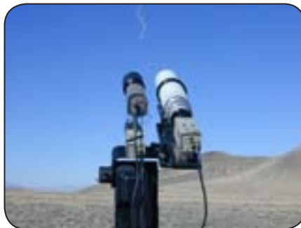
FLIR pan/tilts automatically track missile test flight paths.
