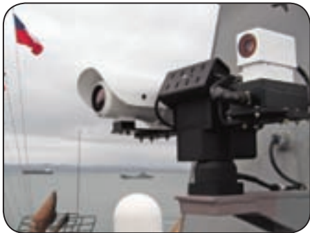
The PTU-300-ISM positioning an Optical Tracker on a Chilean Navy vessel.
