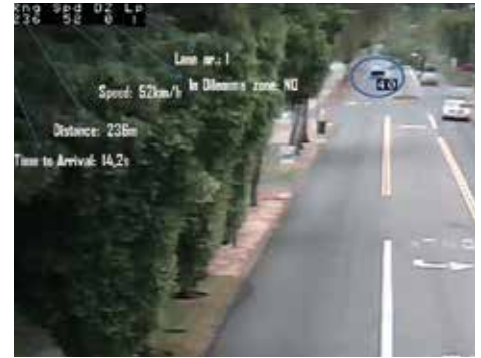
Trafiradar provides accurate data on position per lane, distance and speed, making it an ideal tool for traffic adaptive systems.
