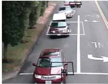
In this example, Trafiradar detects vehicle with ID 27 and 28 to be in the dilemma zone.
