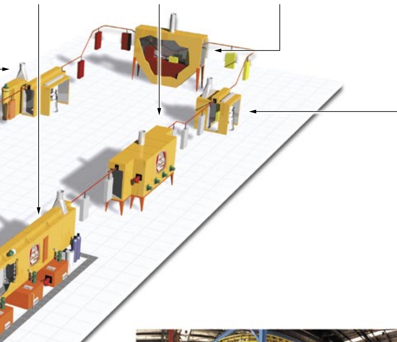
Ets FLUOLUX Pretreatment tunnel Ets BERTHOUD Drying tunnel after pretreatment Ets SCHINDLER Dip-coating paint tank Ets CARLY Spray booth
