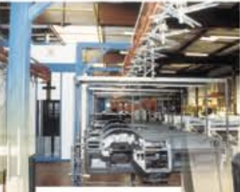
▲ REYDEL - Power and free overhead conveyor with buffer storage
