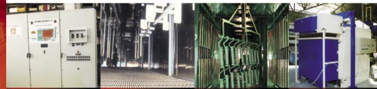
AMC Electric panel control Ets NORPLAST Convection cure oven with floor ducting Ets PEL JOB Infra-red curing oven with gas fired radiant emitters Ets BAYARD Spray booth with built-in cartridge filters
