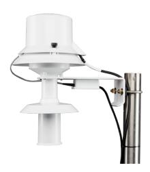
For the upper measurement, attach the 43502 to the top most mast of a UT930 tower (10 m measurement height).
