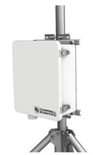
An enclosure mounted to the mast of the CM106.
