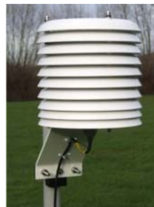
Probe installed in MET20 Radiation Shield
