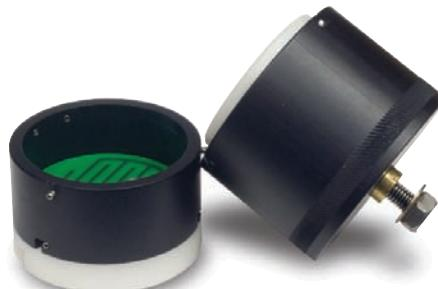
All of the DOT600's components conveniently fit in a rugged case (top photo). Soil is placed in the sample chamber (bottom left) and compacted to a chosen pressure by using the compression cap (bottom right).
