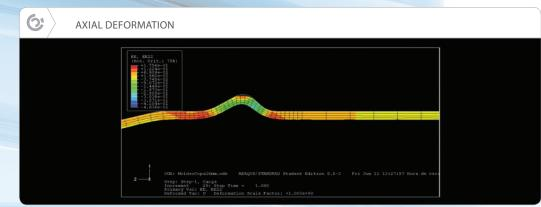
FEM simulation of a PVC-O pipe behaviour with axial and hoop orientation
