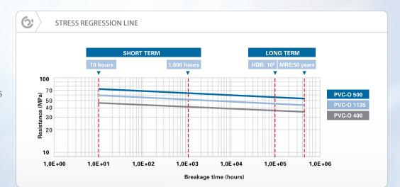
For the American Standards the class should be 1135, according to ASTM D 1483-12. The value is related to the Hydrostatic design Basis (HDB), tested at 10<sup>4</sup> hours and extrapolated to 10<sup>5</sup> hours. Class 1135 means that after 10<sup>5</sup> hours the material withstands at least 6810 psi (46.92MPa).
