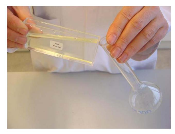
POUR THE 25 ML ALGAL SUSPENSION FROM THE ALGAL STOCK CELL INTO A 100 ML FLASK
