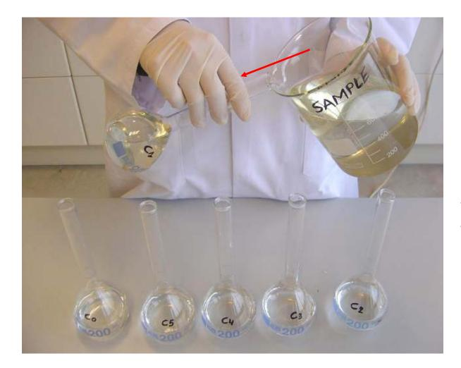
FILL FLASK C1 TO THE 200 ML MARK WITH THE FILTERED SAMPLE
