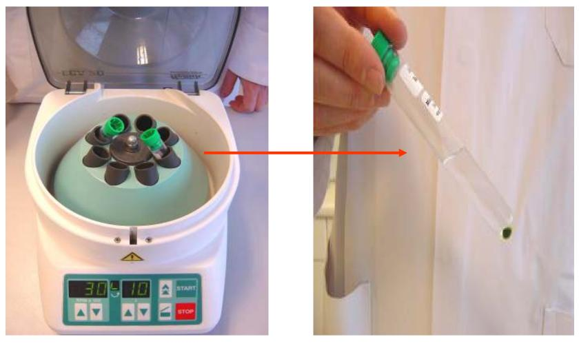
CENTRIFUGE THE TUBE FOR 10 MINUTES AT 3000 RPM IN A CONVENTIONAL LAB CENTRIFUGE
