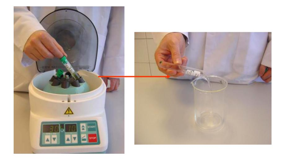
CENTRIFUGE THE TUBE AGAIN AT 3000 RPM FOR 10 MINUTES AND THEN POUR OUT THE SUPERNATANT
