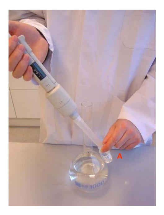
TRANSFER 10 ML FROM ONE OF THE TWO "NUTRIENT STOCK A" VIALS IN ± 800 ML DISTILLED WATER IN THE 1 LITER VOLUMETRIC FLASK
