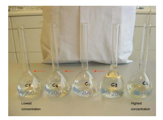
REPEAT THE FORMER DILUTION PROCEDURE FOR THE OTHER FLASKS (i.e., 100 ml from C2 to C3, etc.)
