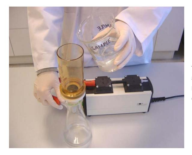
TO ELIMINATE TURBIDITY, SAMPLES MUST BE FILTERED BEFORE TESTING (e.g. over a membrane filter of 0.45 μm),
