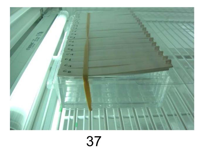
INCUBATE THE HOLDING TRAY WITH THE LONG CELLS FOR 72h IN AN INCUBATOR AT 23°C  $\pm$  2 °C, WITH CONTINUOUS ILLUMINATION:
