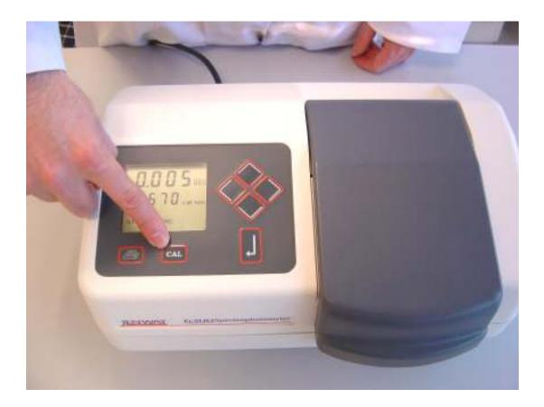
ZERO-CALIBRATE THE SPECTROPHOTOMETER PRIOR TO THE DAILY MEASUREMENT OF THE **OD** IN THE LONG CELLS,
