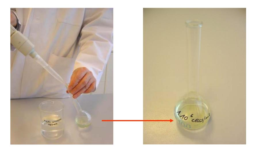
ADD THE CALCULATED VOLUME OF ALGAL CULTURING MEDIUM TO THE FLASK, TO MAKE UP A SUSPENSION OF 1.10<sup>6</sup> ALGAL CELLS / ML
