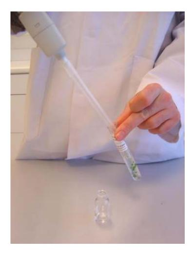
OPEN THE VIAL "MATRIX DISSOLVING MEDIUM" AND TRANSFER 5 ML TO THE TUBE WITH ALGAL BEADS
