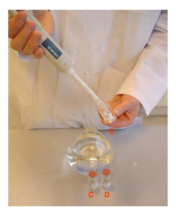
TRANSFER 1 ML FROM THE NUTRIENT STOCK VIALS B, C AND D INTO THE 1 LITER VOLUMETRIC FLASK.
