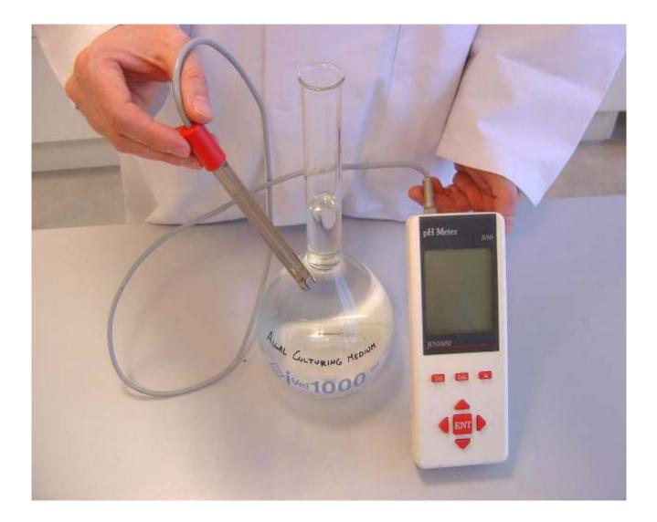
ADJUST THE pH (if necessary) TO 8,1 ± 0,2 (with either 1 M HCI or 1 M NaOH)
