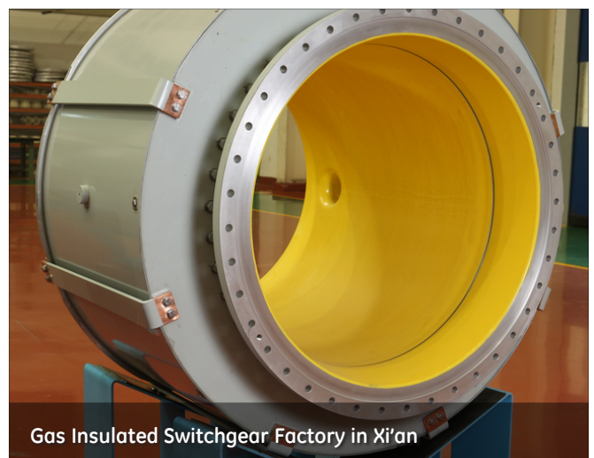
420kV Gas Insulated Switchgear
