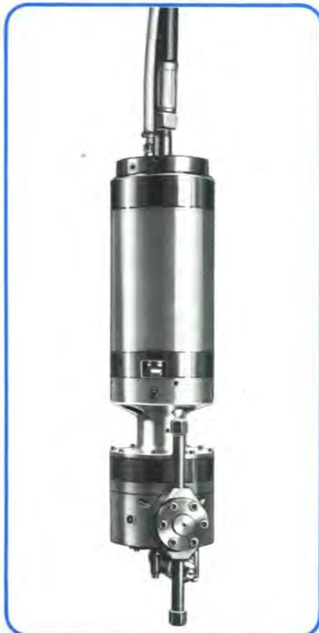
These units basically consist of a head with jets rotating in two perpendicular planes, and a sealed drive motor operating through reduction gears. The head is cycled. The intensity of the cleaning action depends on both available power (flow/pressure) and the number of cycles performed. A built-in indexing system (Barthod patent) provides continuous coverage of the surface to be cleaned and allows an ever closer criss-cross effect of the jet impact lines until the end of the last cycle.
