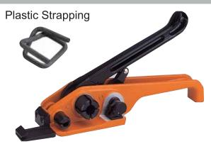
**Strapping Tensioner** with an extended nose section, designed to tighten 12m to 19mm PET and Polywoven/ Cord strapping. Specically for use with 12mm, 16, and 19mm wire buckles.
