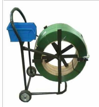
**Mobile Strap Dispencer for plastic band** with seal tray and adjustable inner core diameter.
