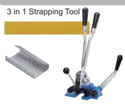
**Combination tool** (tensioning, sealing and cutting all in one) for PP strapping (12.5 - 1.6mm) 16mmPP/PET. Use with CP04 seals.
