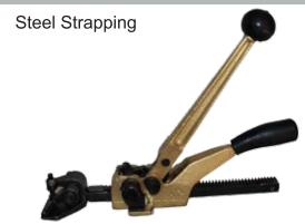
**Heavy Duty Rack Tensioner** capable of tensioning straps ranging in widths from 16-32mm width and 0.5 to 0.9mm thickness Steel Strapping. Ideal for Circular Applications.
