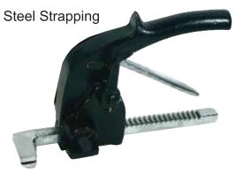
**Rack-Type Pusher Bar Tensioner** capable of adjusting straps ranging in widths from 10-13mm 0.38 to 0.6mm Steel Strapping. Ideal for Circular Applications.
