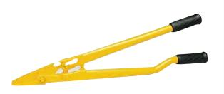
**Heavy Duty Steel Strap Cutter** SAE 4140 high carbon steel drop forged heavy duty steel strapping cutter for straps up to 2" x 0.05". 24" Handles
